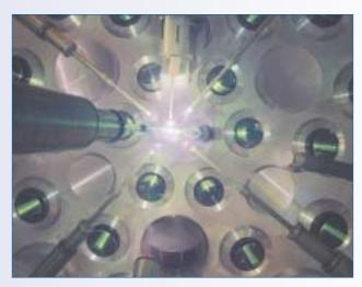
THE UNIVERSITY OF ROCHESTER Laboratory for Laser Energetics uses OSLO extensively in the development of its Omega laser. Currently the world's most powerful system for studying laser fusion, the Omega laser uses hundreds of optical components to split and amplify a nanosecond, millijoule optical pulse to more than 30,000 joules that are focused uniformly on a tiny deuterium pellet.
