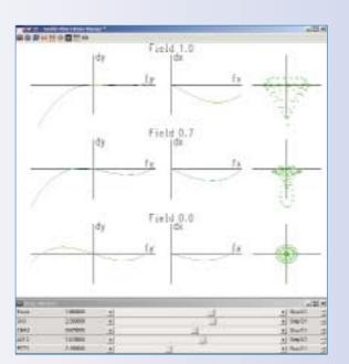
OSLO'S HIGH-SPEED GRAPHICS SUBSYSTEM provides interactive design windows that allow you to attach graphical sliders to lens parameters and see the performance change instantly as the sliders are dragged. In this tutorial example, the Seidel aberrations are adjusted with the sliders and the performance curves are updated dynamically. OSLO allows you to carry out complete optimization iterations while dragging a slider.
